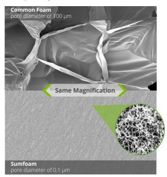
Pore size smaller by factor 1,000 compared to conventional foams.
