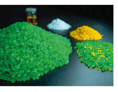
Particularly applicable in the rubber and plastics industry, Sumfoam enables functional liquids to be absorbed and makes them available as dry liquid for the extrusion or injection molding process.
